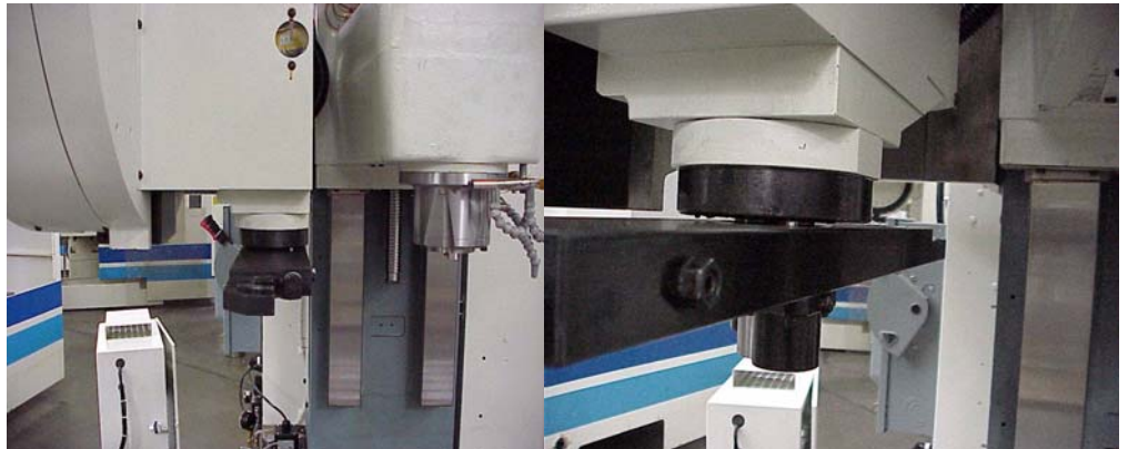
Figure 7-24: Place Taper Lock and Arm Assembly into Tool Changer Spindle
