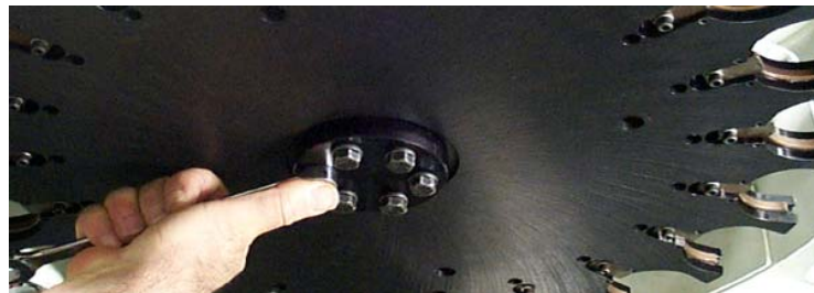
Figure 7-7: Loosen Hex Bolts Holding Tool Carrier
