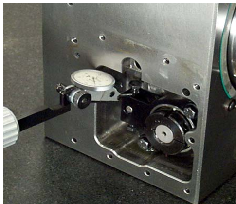
Figure 8-7: Zero Indicator on Worm Pivot Plate
