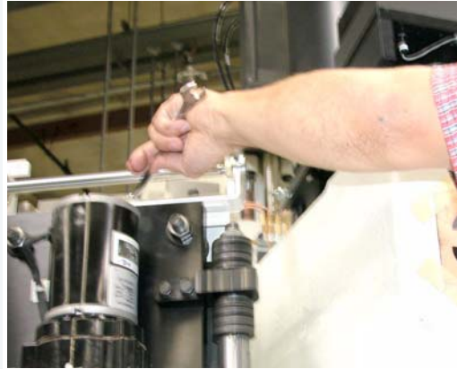
Figure 7-5: Loosen Hex Bolts / Move Slide to Spindle Until Engaged
