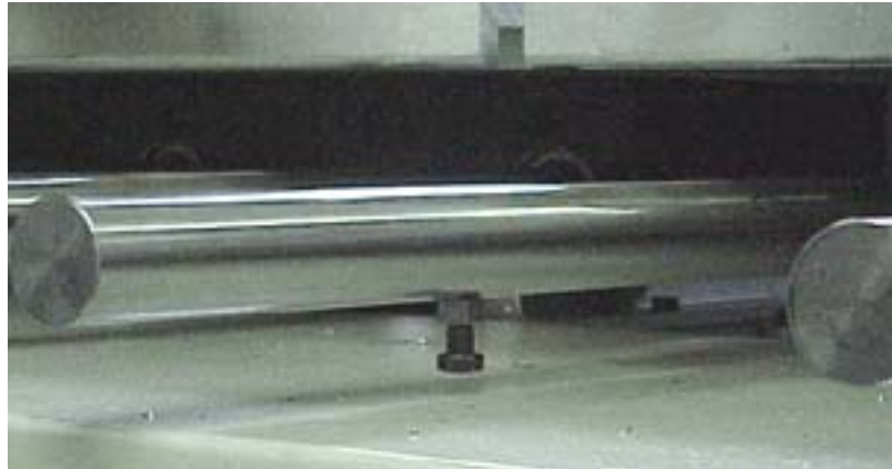
Figure 9-1 Verify Rail Support Bolts are Installed and All the Way Up
