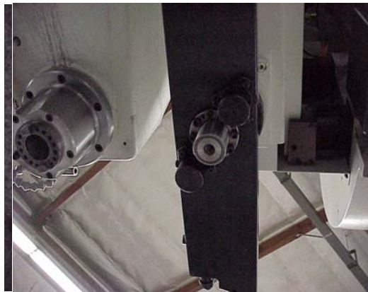
Figure 7-25: Insert and Tighten Installation Tool
