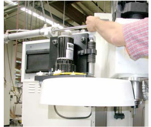
Figure 7-5: Loosen Hex Bolts / Move Slide to Spindle Until Engaged
