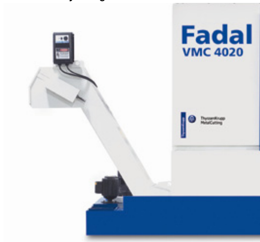
Figure 3-15 Conveyor Against Left Side of Sheet Metal
