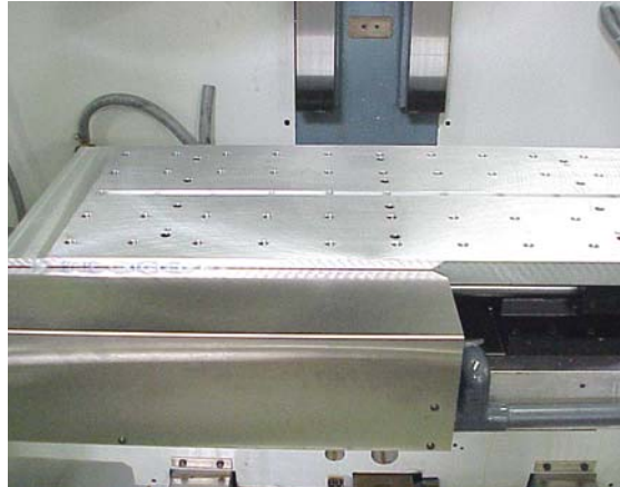
Figure 9-3 Remove Pallet Arm Safety Cover
