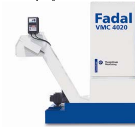
Figure 3-15 Conveyor Against Left Side of Sheet Metal
