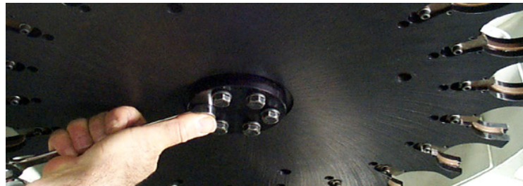
Figure 5-6 Loosen Hex Bolts Holding Tool Carrier
