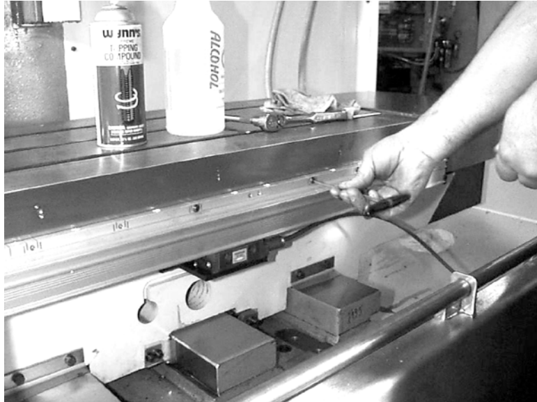
Figure 11-21 Attach Scale Assembly to Table
