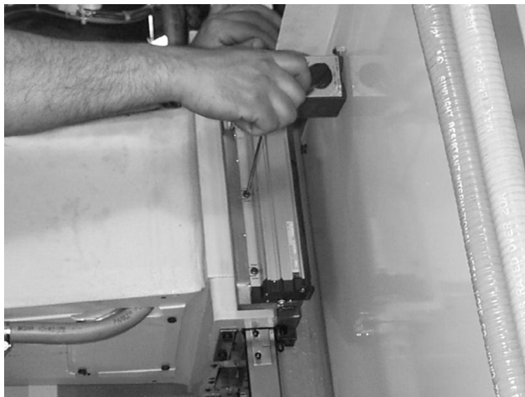
Figure 11-68 Attach Scale to Mounting Plate
