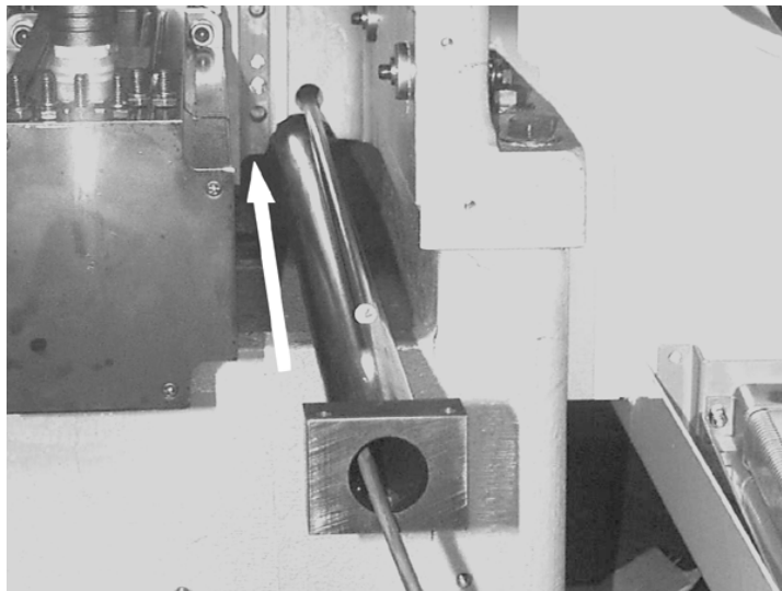
Figure 11-32 Insert Tube Through Column
