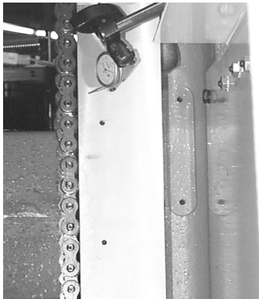
Figure 11-61 Mount Dial Indicator to Column
