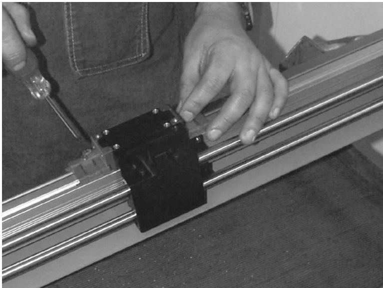
Figure 11-38 Remove Packing Clips from Scale Assembly
