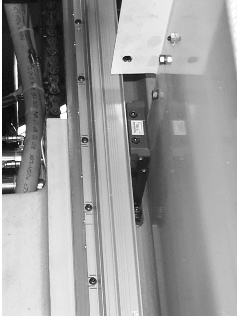
Figure 11-71 Attach Scale Reader to Mounting Bracket
