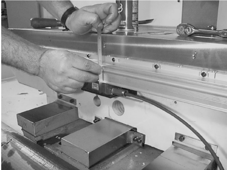
Figure 11-25 Adjust Reader So it is Flush with Scale
