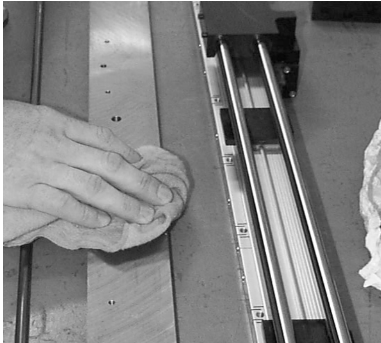
Figure 11-63 Thoroughly Clean Z Axis Mounting Plate
