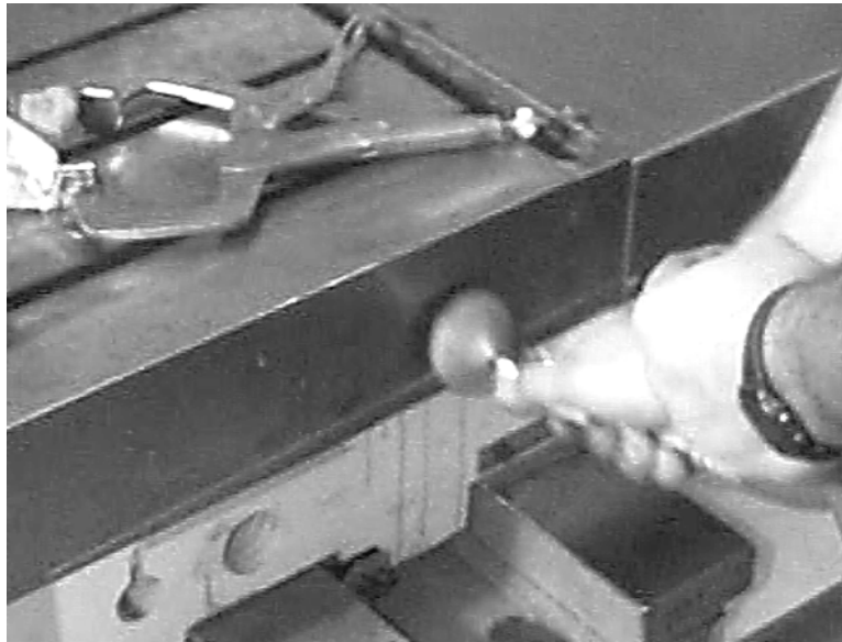
Figure 11-11 Clean Debris from Holes
