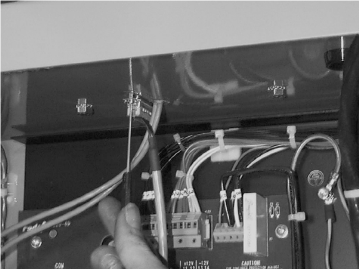
Figure 11-101 Plug 15 Pin Connector into Scale Box Connector
