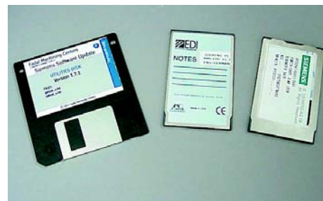
Figure 7 The files for performing the MMC100 software update are stored on two PC cards and Utilities disk.
