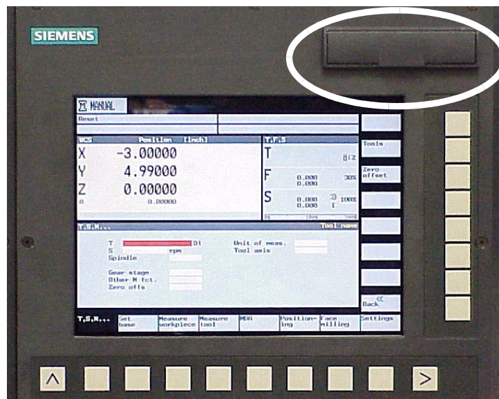
Figure 17 The PC card is inserted into the card slot of the operator panel for the HMI firmware installation.
